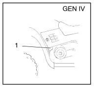
**NOTE:** Some coolant level drop on new machines is normal, as the system is purging itself of trapped air. Observe coolant levels and maintain as recommended by adding coolant to the recovery bottle.
